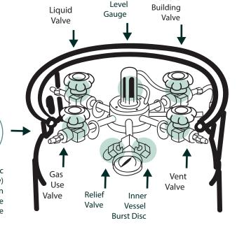
Vacuum Burst Disc (Detail view) Located between Liquid and Gas Use Valve
