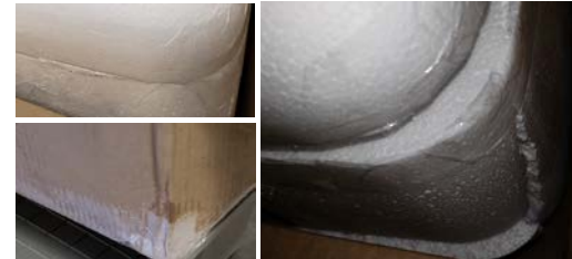
Figure 1. This insulated chest containing dry ice was received completely sealed with tape. The build-up of pressure ruptured the side of the chest and allowed for the formation of frost on the outer packaging.
