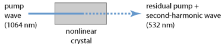
Illustration of a typical configuration for frequency doubling: an infrared input beam at 1064 nm generates a green 532 nm wave during its path through a nonlinear crystal.
