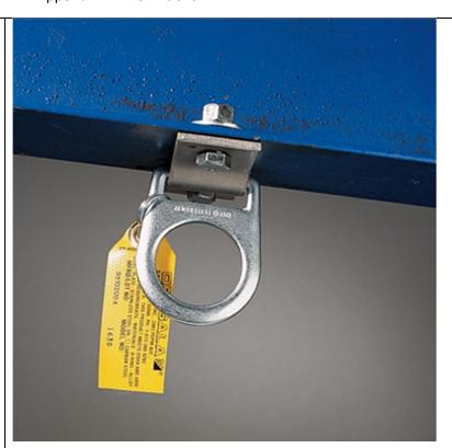
Anchorage Connector- A component of subsystem that functions as an interface between the anchorages and fall protection, work positioning, rope access or rescue system for the purpose of coupling the system to the anchorage.
