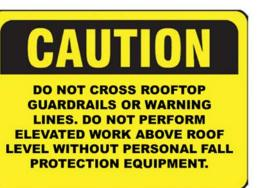
This CAUTION sign shall be placed on all permanent point(s) of access to any roof area. Consult with PMCS as to proper placement and attachment of signs.
