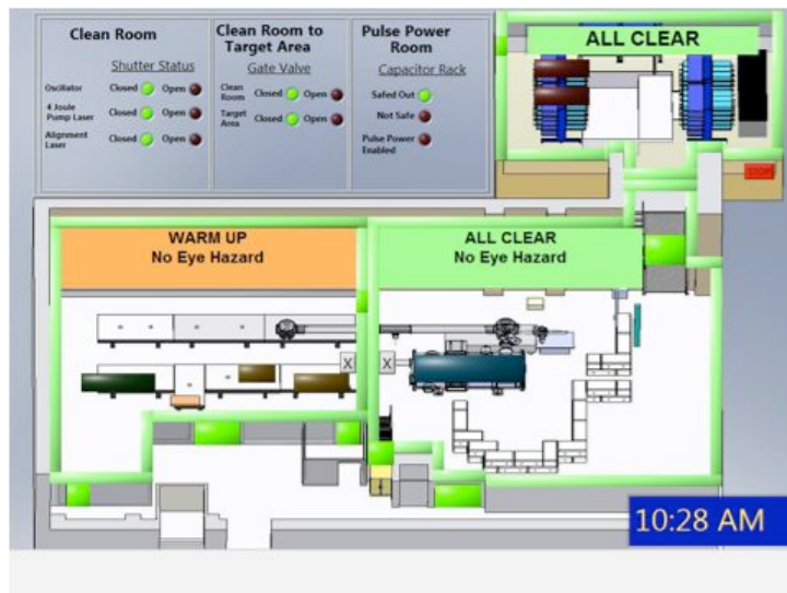
Figure 5. Status panel configuration for indicating the laser is in WARMUP mode.
