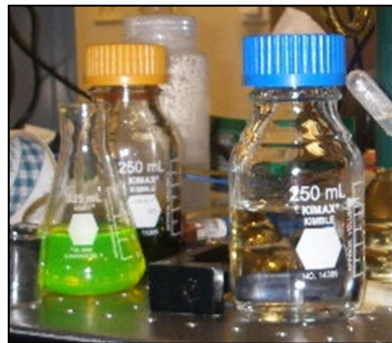
Improperly labeled secondary storage container
