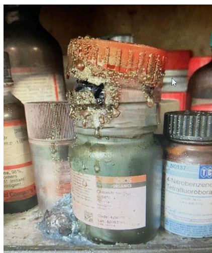
Poor Chemical labelling and Container Condition
