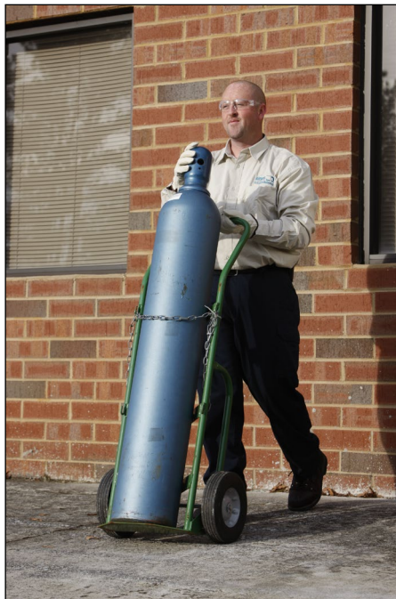
Proper transport of gas cylinders (picture courtesy of Airgas, Inc)
