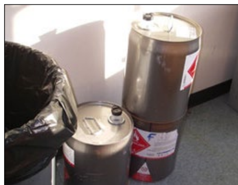
Improper storage of flammable chemicals
