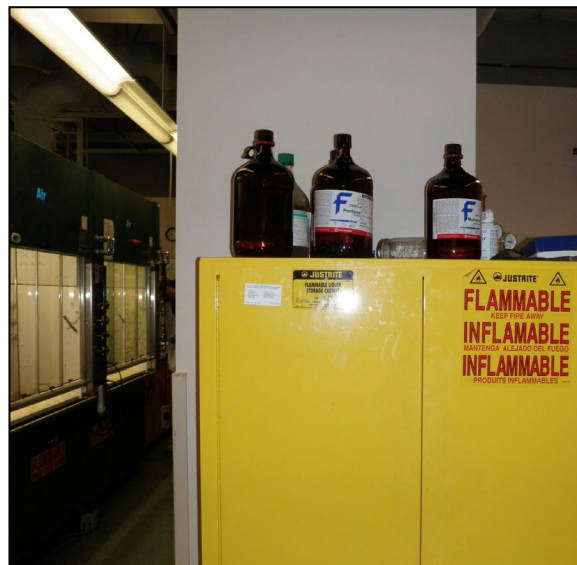
Improper storage of chemicals above eye level
