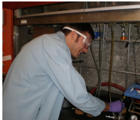
Improper use of the fume hood.
