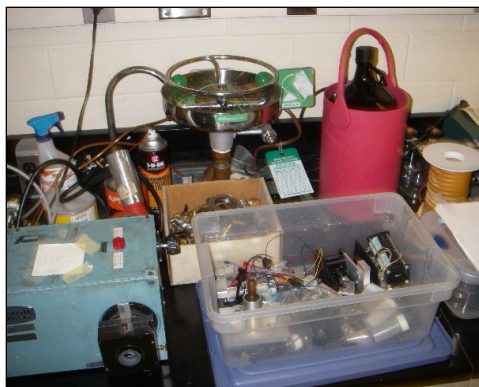
Cluttered workspace. Emergency eyewash obstructed
