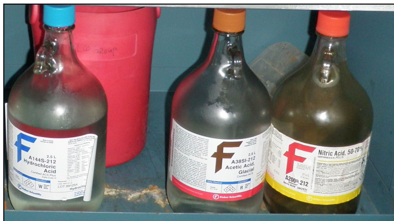
Improper storage of nitric acid
