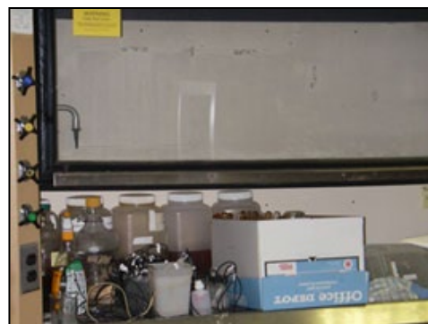
Improper storage in a fume hood
