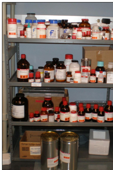
Proper storage of chemicals below eye level
