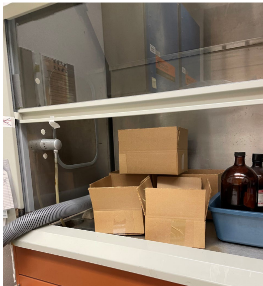
Do not store chemicals or other items in the fume hood.
