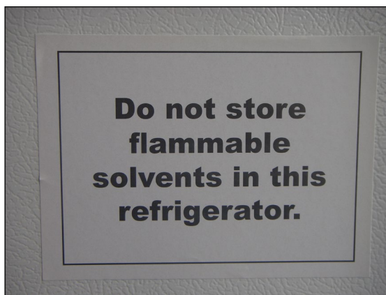
Refrigerator warning label when not rated as intrinsically safe
