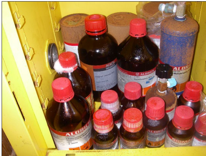
Chemical containers in poor condition from corrosion and crystal formation
