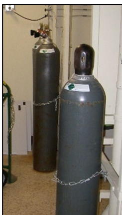
Acceptable method of securing a gas cylinder
