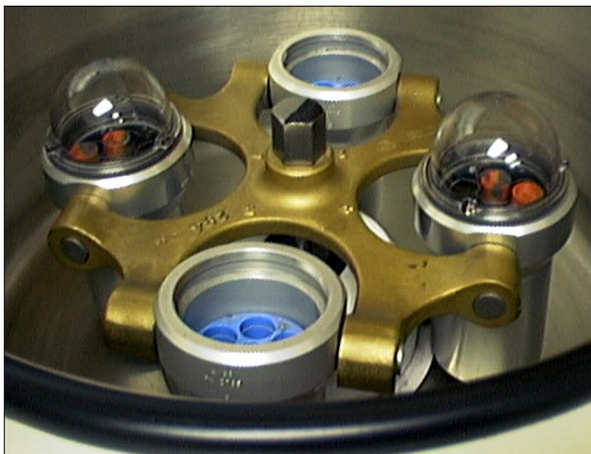
Sealed safety cups being used in a centrifuge.
